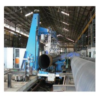
The Spiral-Saw UT test systems is to test the Weld defects based on the International Standard in general API, Shell, Etc.The Test Mechnism will have probe carriege shall be in number 2 to 4 based on the test configration Mode like nos of I-mode, X-mode, Tendom, HAZ, Onbead, etc. Additional can be provided the edge testing arrangement in the system.
